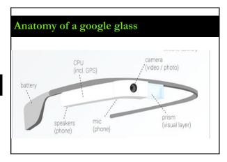
the device as light as possible, most of the processing actually takes place in the cloud. Thus, a good mobile broadband signal is essential for google glass to remain operative.
